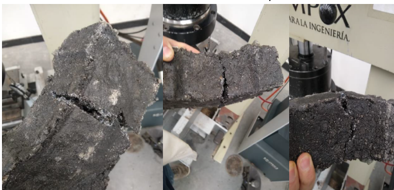
Figure 8 Failure to the middle third of the specimen
